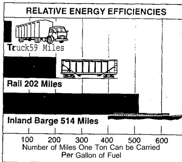
This modal comparison of fuel consumption on a ton-mile per gallon basis reveals that a semitrailer on the highway carries somewhat less than 300 pounds per horsepower; a 175-car trainload of iron ore carries about 4,500 pounds per horsepower; and a 5,600 horsepower towboat is capable of propelling some 30,000 tons of cargo, which is equivalent to about 10,700 pounds per horsepower. 5/
